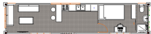
40 ft refurbished container converted into a one-bedroom open-plan home, with flexibility to be adapted into a two-bedroom layout.
